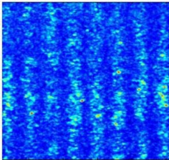
Stripyness in print: uneven print on flute valleys compared to flute tips, this can be caused by mechanical wash boarding but also by other peripheral circumstances.
