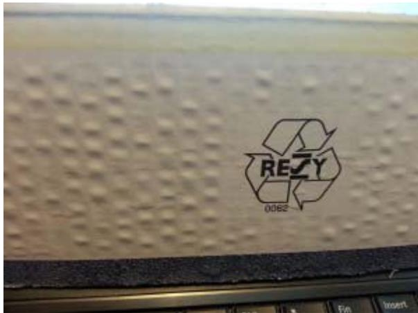
Cockling or honeycomb: too high moisture will cause the fibres to expand. This will happen in proportion a lot more in the width than in the length. The fibre direction of the liner is always perpendicular to the flutes.
