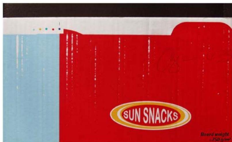
Stripyness caused by post glazing: the corrugating process is a physically very rough process. Take a coated liner, moisten it, heat it and then drag it for about 15 meters under high pressure on metal heated plates. This can and will change the coating structure on the flute tips and will result in a different way how inks are settling or penetrating. You can compare post glazing with what happens if you iron the pants of your best suit too warm...your pants start to shine.
