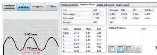
Incorrect flute profiles are one of the key parameters for **STRIPYNESS** in flexo post print.
